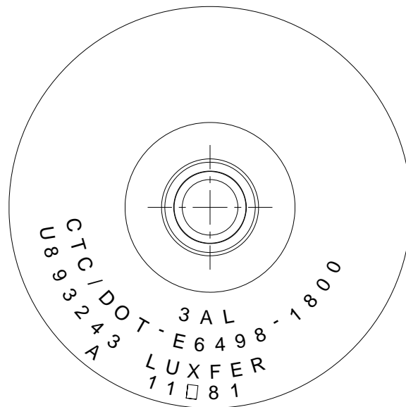
Figure 2—3AL marked exemption cylinder
