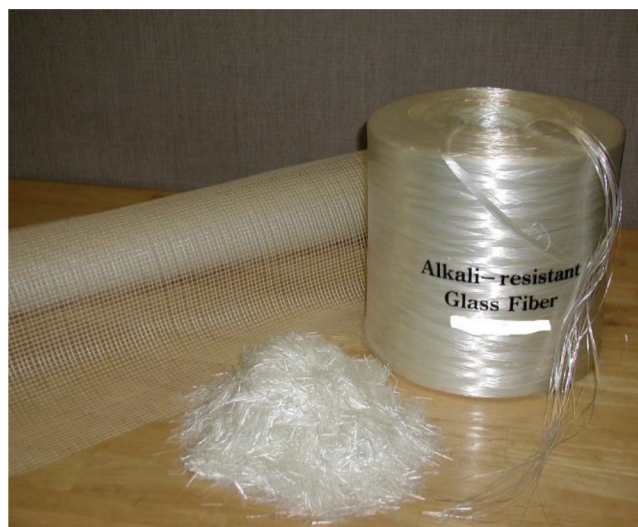
Fig. 1.1—Alkali-resistant glass fiber roving, chopped strands, and textile (bonded scrim).
